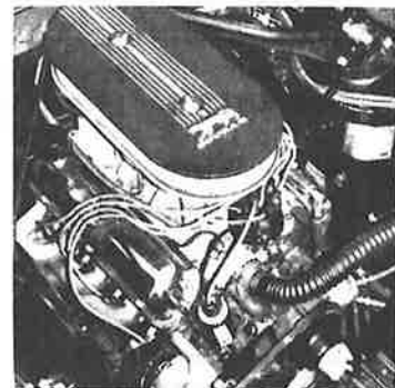
Spring-tower strut installation is sanitary, prevents camber change under stress conditions.
