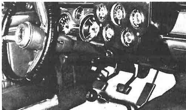
Direct-reading instruments include (l. to r.) transmission oil temperature, tach, engine oil temperature, oil/fuel pressures.
