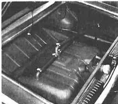
37-gallon fuel tank is assured of ambient pressure by this extra-large vent.
