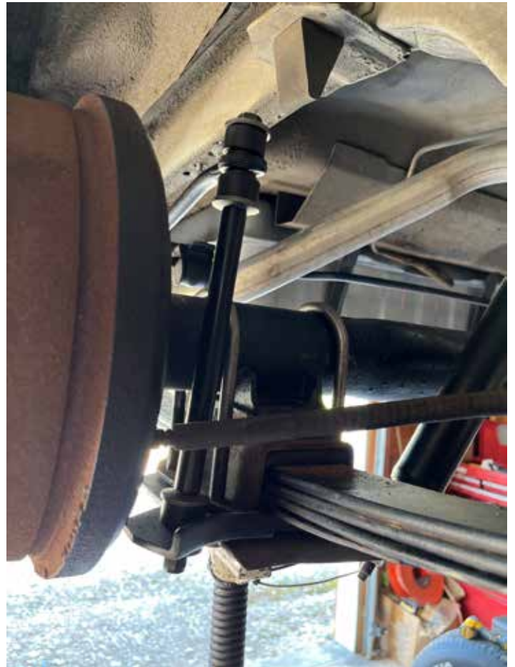
Rear sway bar equipped on all Cougars with the GT package and Q code vehicles, equipped with the " cobra jet performance group package
